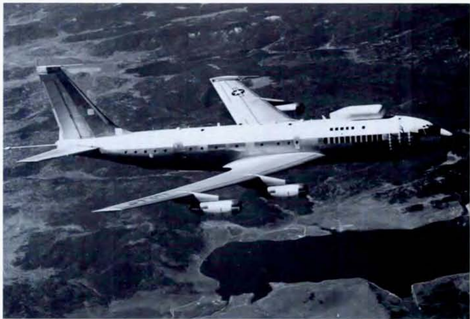
The USAF NC135A-369 containing the Los Alamos Airborne Diagnostics Laboratory. This plane, part of the atmospheric test readiness program, was available and ready to measure device performance in the event that atmospheric testing was resumed. Used during the 1960s and 1970s for several test readiness exercises and numerous purely scientific missions (solar eclipse, cosmic ray, auroral, and other), this plane is now retired.
